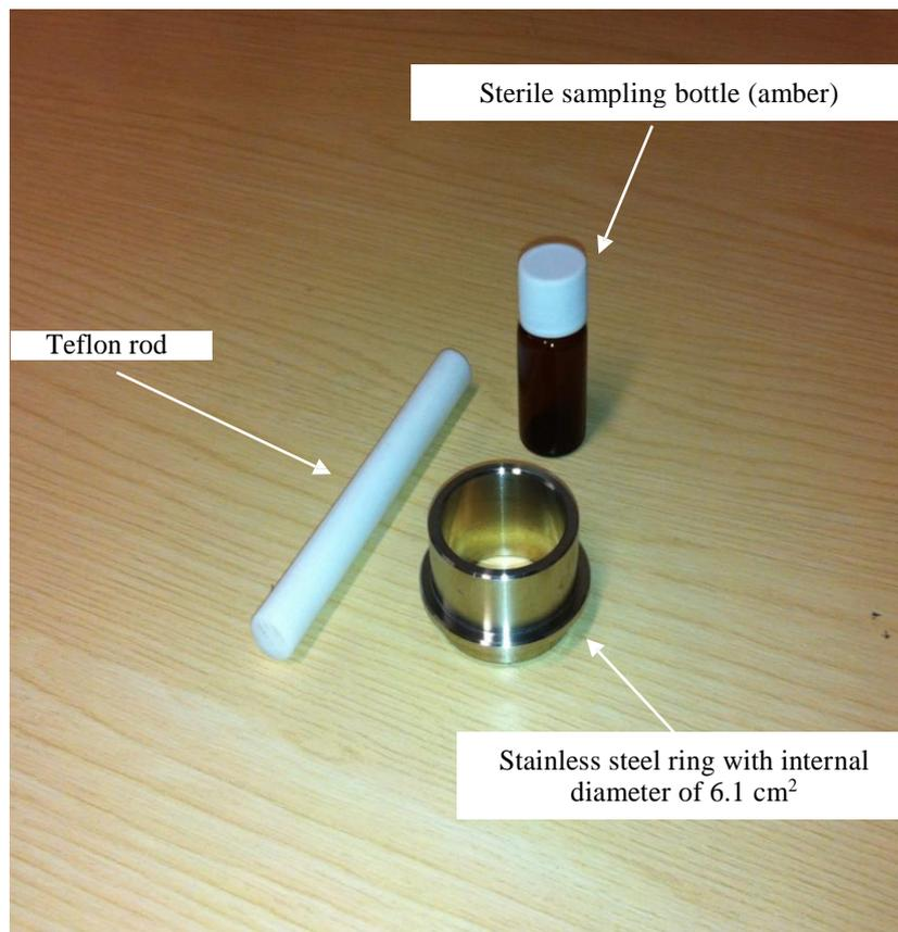
**Figure 4.7:** Instruments used for sampling cutaneous microflora using the surface scrub technique of Williamson and Kligman.
