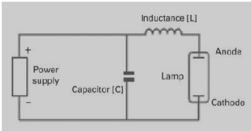
**Figure 3.2:** Circuit diagram for a flashlamp power supply. *Adapted from Ash et al. [211].*
