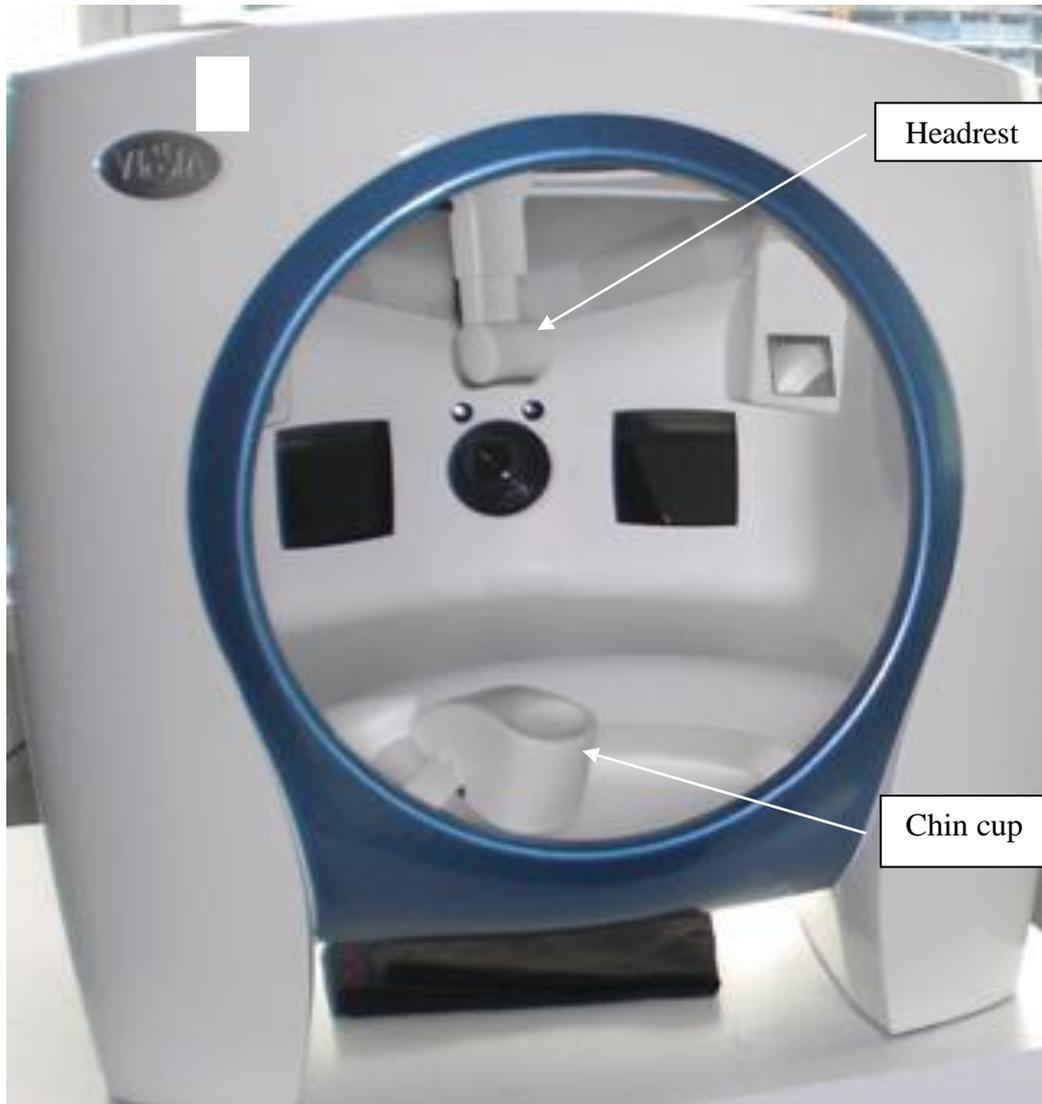
**Figure 4.6:** The Canfield VISIA® Complexion Analysis system consisting of a booth, chin cup and headrest.
