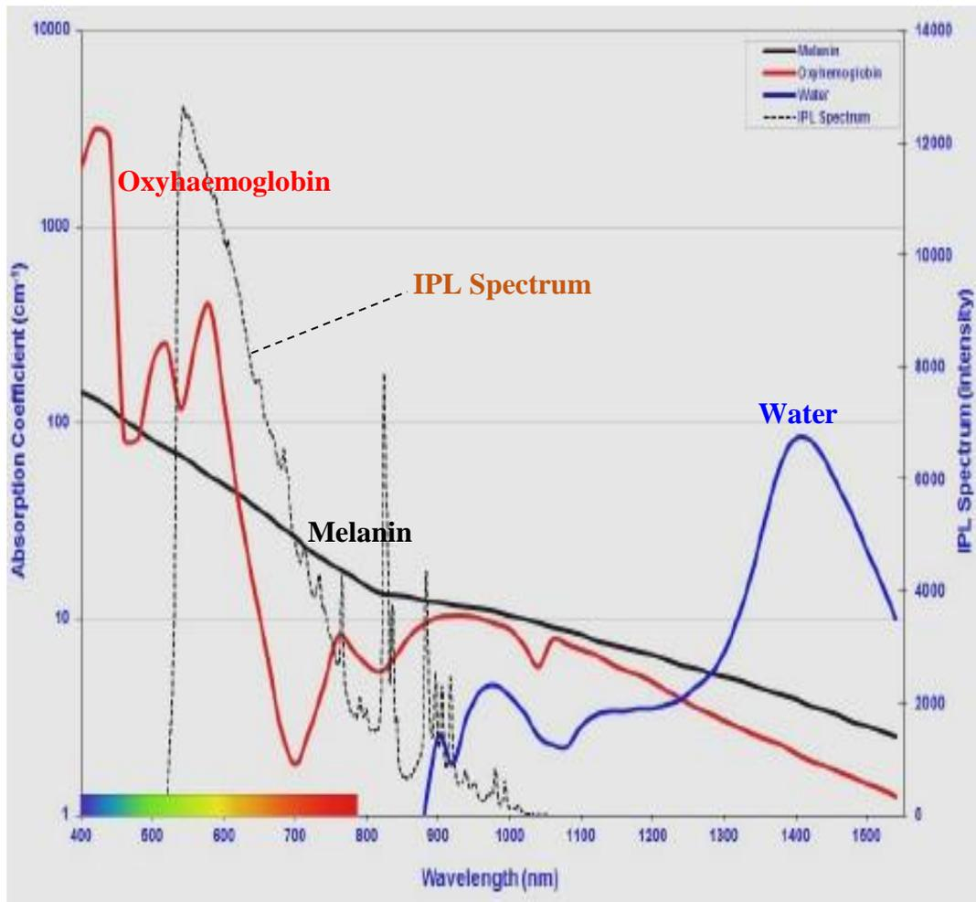
**Figure 3.1:** Absorption coefficients of melanin, oxyhaemoglobin, and water. The emission spectrum of an IPL device has been overlaid. *Adapted from Ash et al. [209].*
