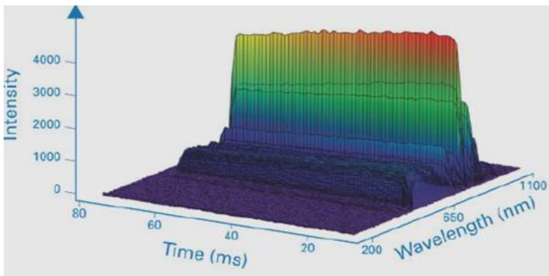
**Figure 3.4:** Time-resolved spectral output image of a single pulse constant current IPL device (*iPulse*, Cyden Ltd), with a measured total pulse duration of 50 ms, producing a constant optical discharge throughout the pulse. *Adapted from Ash et al. [211].*
